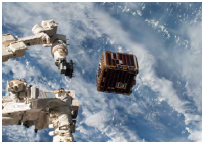
Deployment of the NanoRacks-Remove Debris Satellite from the International Space Station (ISS) using the NanoRacks Kaber MicroSat Deployer. NanoRacks-Remove Debris aims to demonstrate key technologies for Active Debris Removal to reduce the risks presented by space debris.
