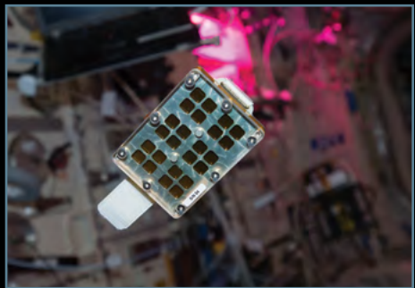
The Microbial Aerosol Tethering on Innovative Surfaces in the International Space Station (MATISS) experiment investigates the antibacterial properties of materials in space to see if future spacecraft could be made easier to clean. The experiment aims to understand the mechanisms of attachment of biofilms in microgravity conditions.
