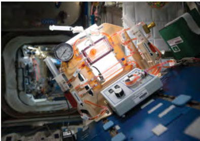
The Capillary Structures for Exploration Life Support investigation studies water recycling and carbon dioxide removal using structures of specific shapes to manage fluid and gas mixtures, benefiting future efforts to design lightweight, more reliable life support systems for future space missions.
