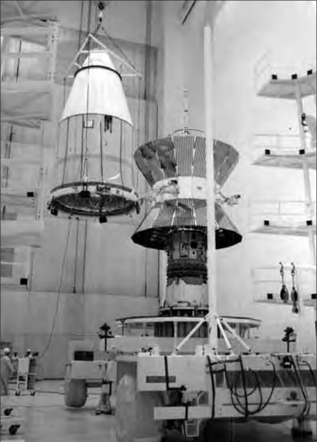
*A Helios spacecraft prototype is encapsulated in its payload fairing at Kennedy Space Center on 27 September 1974. This work was in preparation for a future Titan-Centaur flight. (NASA KSC\_74P\_0222)*
