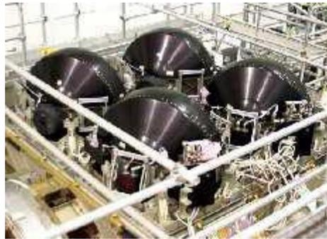
*Z1 truss will house four CMGs (above) that will provide ISS attitude control*
