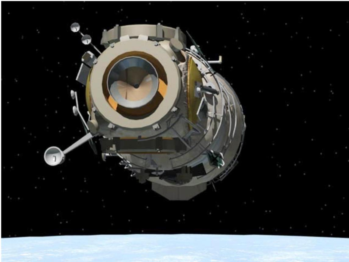
*An automatic sequence of computer commands on Zvezda will order deployment of antennas for its Kurs rendezvous and docking system, and for the Lira communications system*
