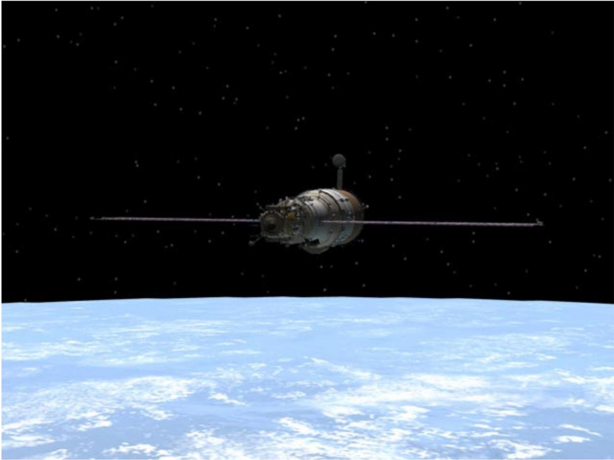
*A day prior to docking, Zvezda will be maneuvered to its docking orientation and its solar arrays moved into the proper docking position, to verify any impact that orientation will have on battery charging*
