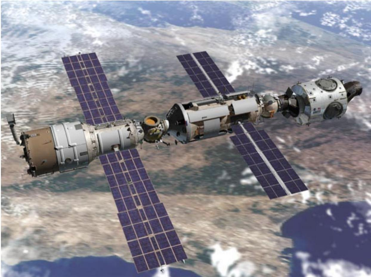
*With the Zarya module controlling, the station will chase and catch up to Zvezda. Ground commands through Zarya's automated rendezvous system, will slowly pull the station next to the module, and then capture Zvezda*
