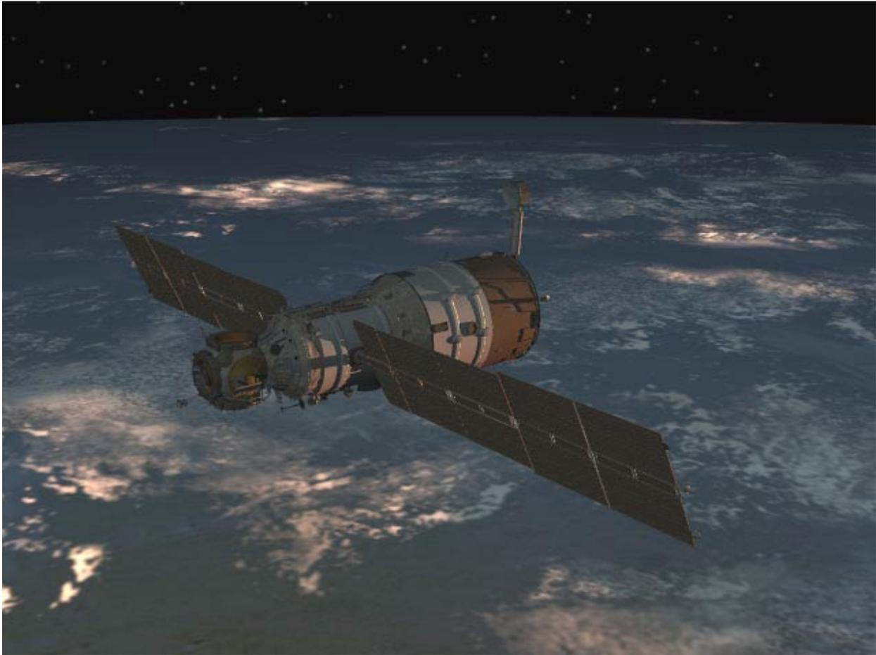
*Over the course of the next several days, controllers will first test the ability of the module's motion control system to orient the solar arrays while flying in darkness, and then test the efficiency of the solar arrays themselves. They will also verify telemetry to and from the motion control system computer to ensure that Zvezda is ready to meet ISS*
