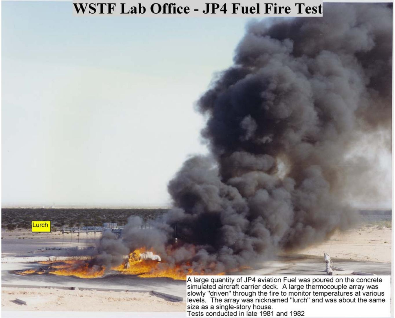
A large quantity of JP4 aviation Fuel was poured on the concrete simulated aircraft carrier deck. A large thermocouple array was slowly "driven" through the fire to monitor temperatures at various levels. The array was nicknamed "lurch" and was about the same size as a single-story house.
