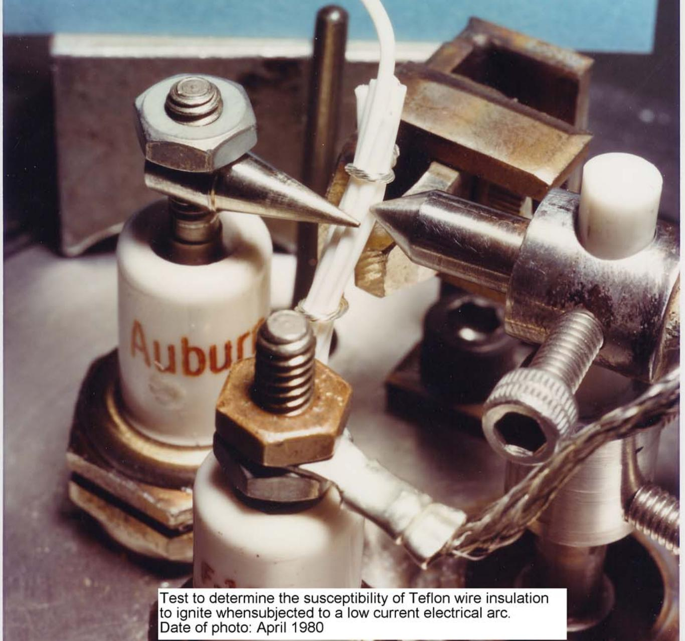
Test to determine the susceptibility of Teflon wire insulation to ignite when subjected to a low current electrical arc.
