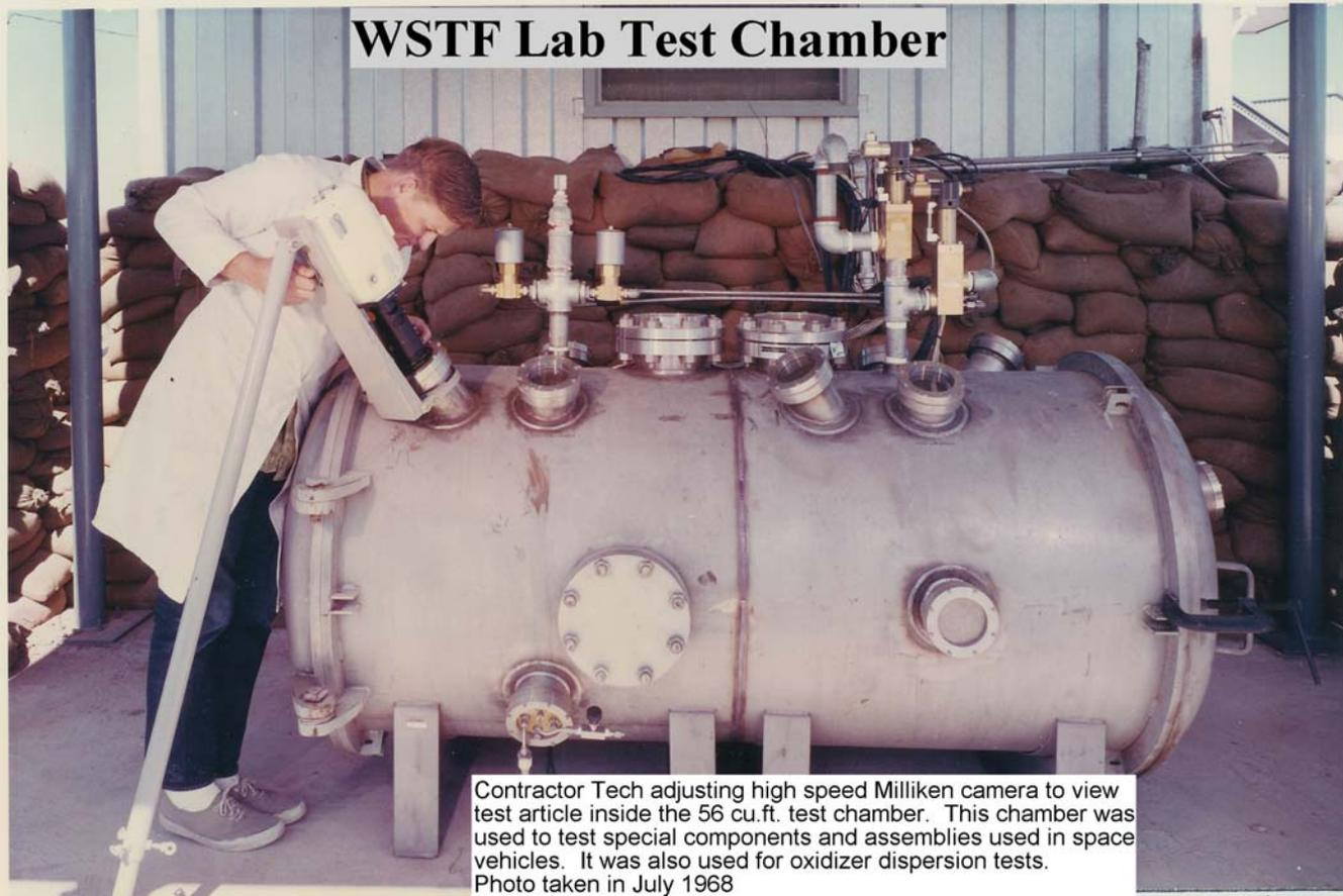
Contractor Tech adjusting high speed Milliken camera to view test article inside the 56 cu.ft. test chamber. This chamber was used to test special components and assemblies used in space vehicles. It was also used for oxidizer dispersion tests. Photo taken in July 1968
