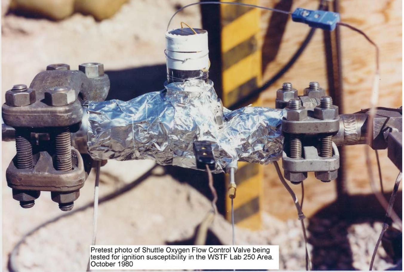
Pretest photo of Shuttle Oxygen Flow Control Valve being tested for ignition susceptibility in the WSTF Lab 250 Area. October 1980
