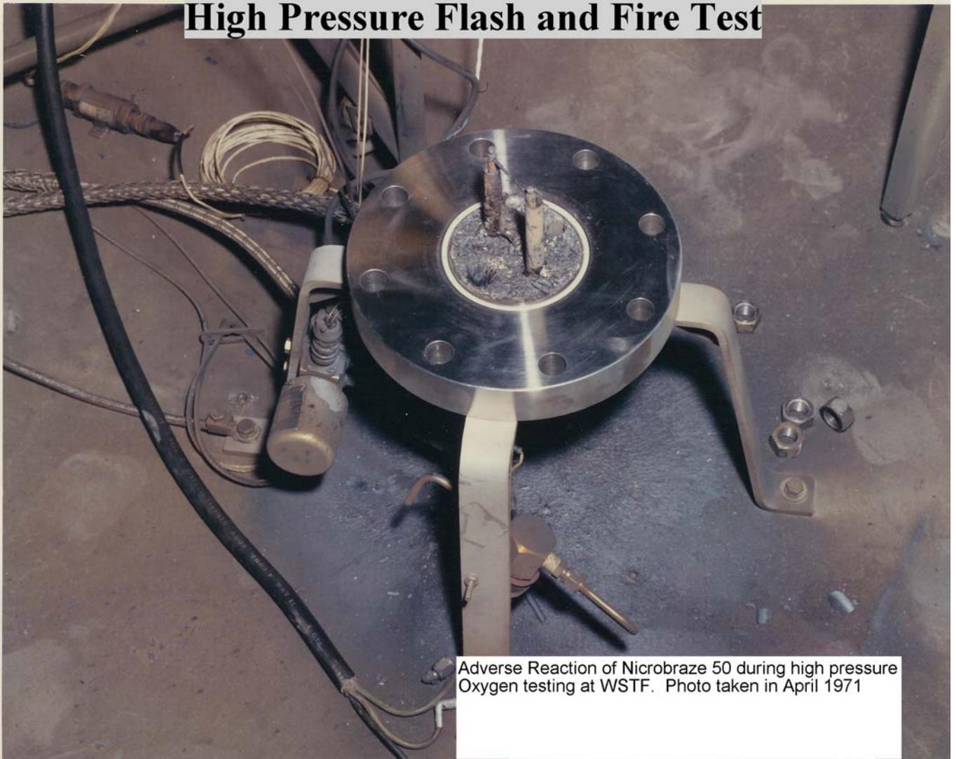
Adverse Reaction of Microbraz 50 during high pressure Oxygen testing at WSTF. Photo taken in April 1971
