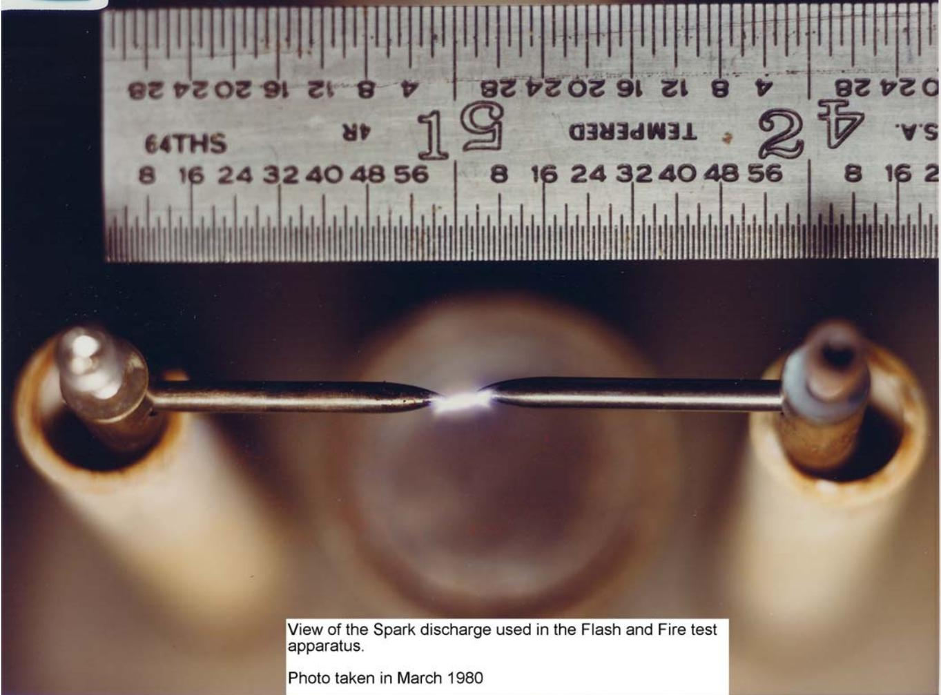
View of the Spark discharge used in the Flash and Fire test apparatus.
