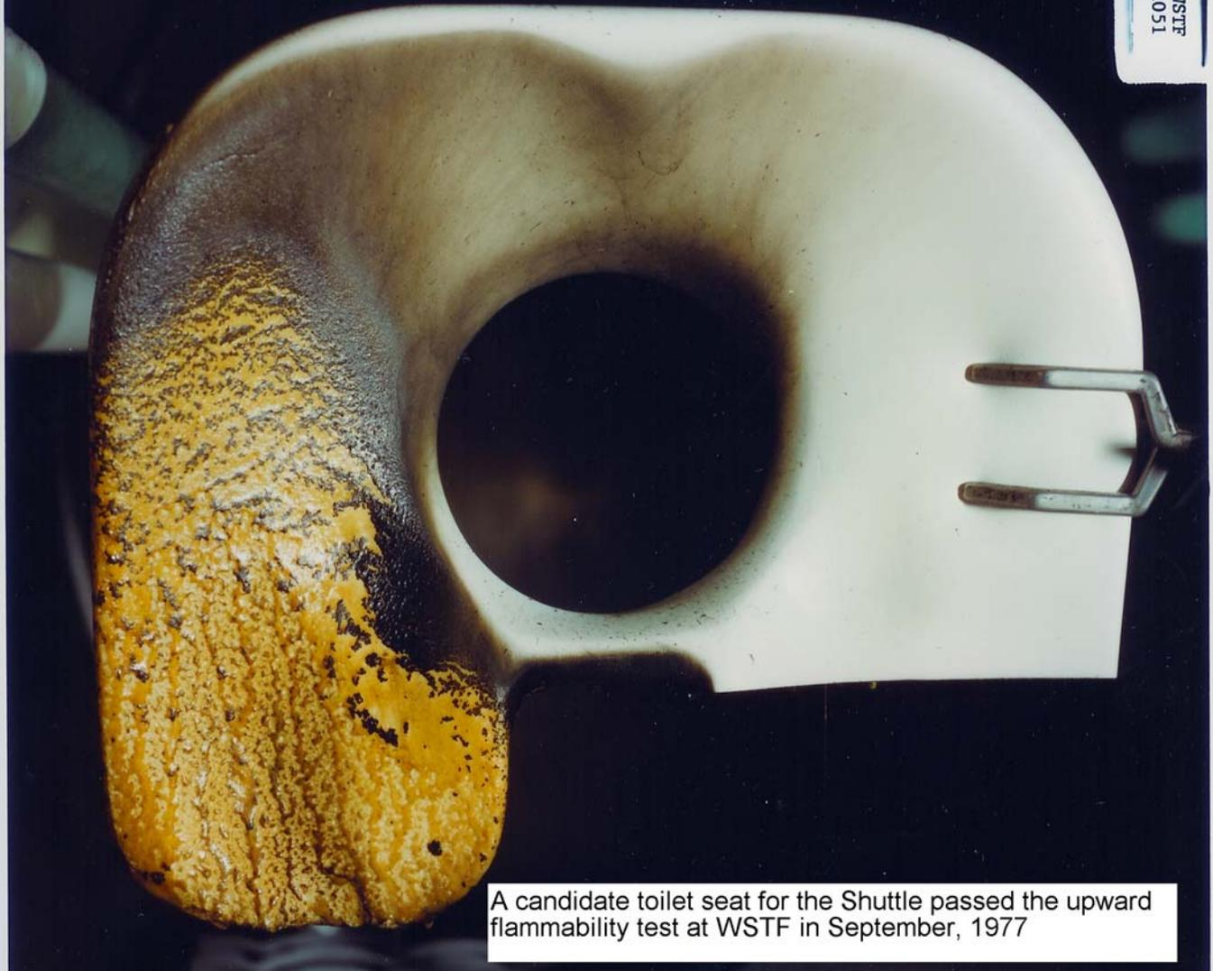
A candidate toilet seat for the Shuttle passed the upward flammability test at WSTF in September, 1977
