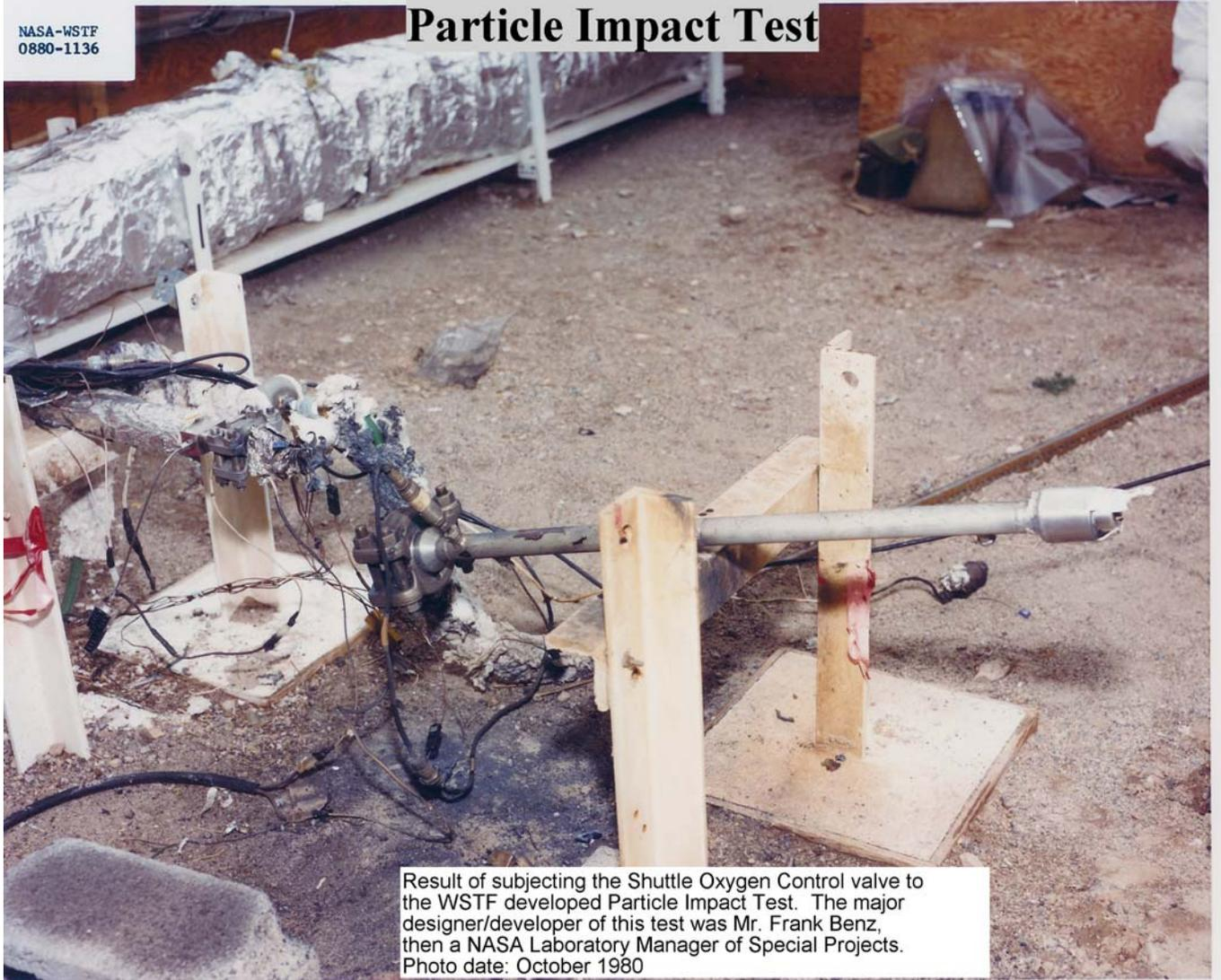
Result of subjecting the Shuttle Oxygen Control valve to the WSTF developed Particle Impact Test. The major designer/developer of this test was Mr. Frank Benz, then a NASA Laboratory Manager of Special Projects. Photo date: October 1980
