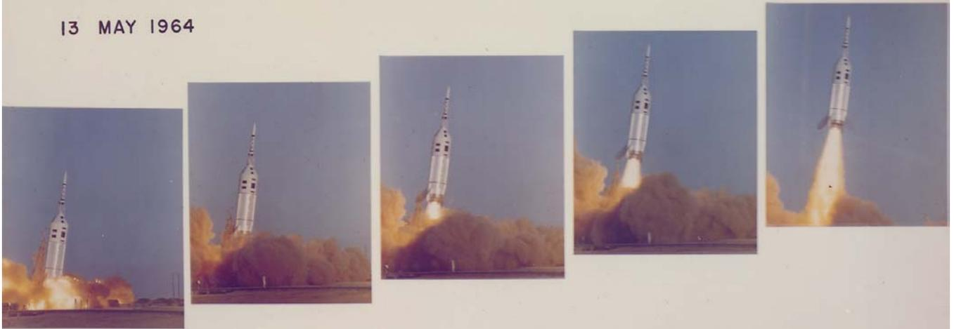
*Photo A-13 - Sequence of photographs of BP12 that occurred on May 13, 1964. The lower sequence of events shows the launch and the top sequence of events shows the launch escape system pulling the command module from the booster.*
