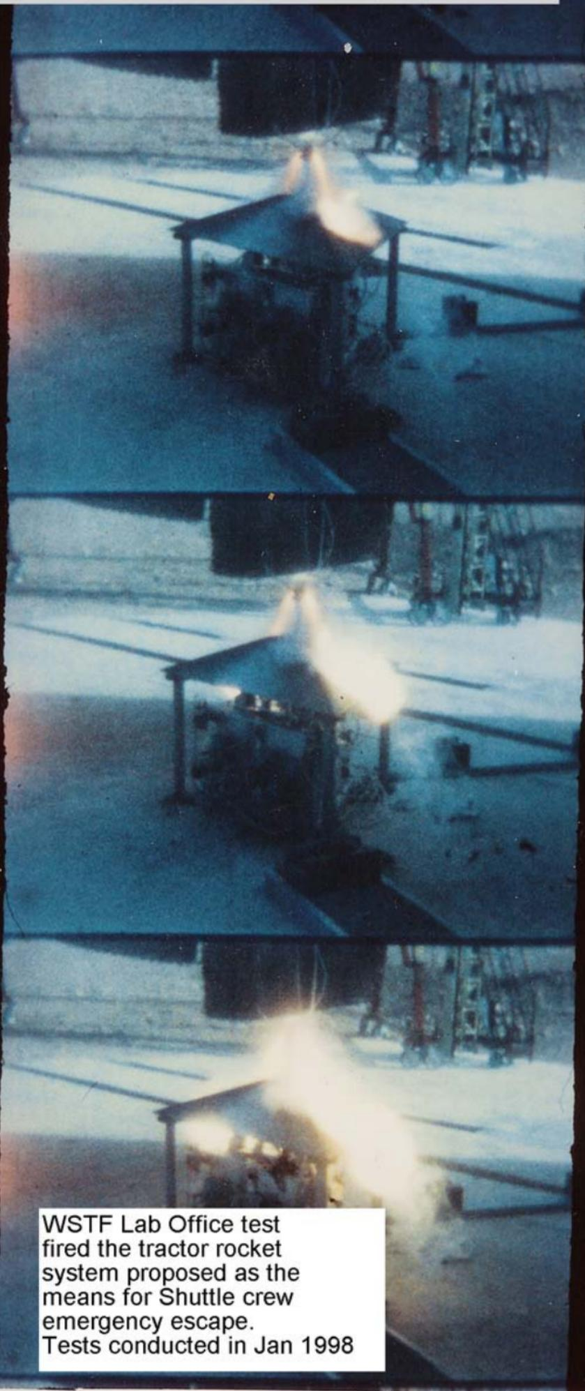
WSTF Lab Office test fired the tractor rocket system proposed as the means for Shuttle crew emergency escape. Tests conducted in Jan 1998
